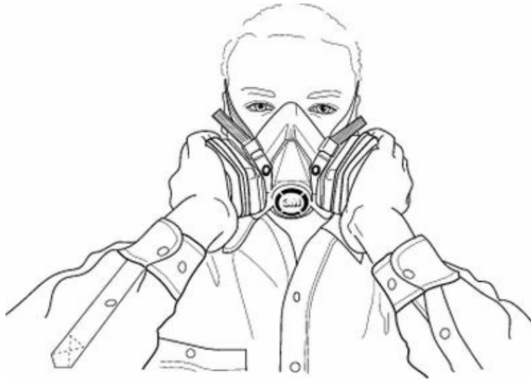
Example of Negative Pressure Seal Check for reusable respirator. Place the palms over the cartridge and inhale gently. The respirator should collapse slightly. (Refer to manufacturer's guides)
